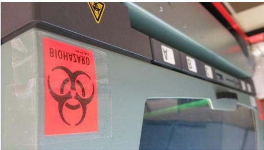
Samples of deer brain and lymph nodes are soaked in formaldehyde, then dehydrated with alcohol, saturated with paraffin wax, and shaved into slivers just five microns thick. This machine runs the samples through a bath of red dye, which only sticks to the misfolded proteins, called prions, that cause chronic wasting disease. John Enger | MPR News
